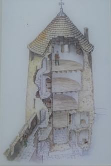
A cut-away view of the Lady Tower. (Illustrated by Philip Corke).
